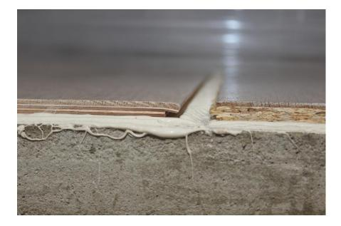
After the end of the experiment, when the air humidity had decreased to 30 %, gaps were observed between individual floor boards.
